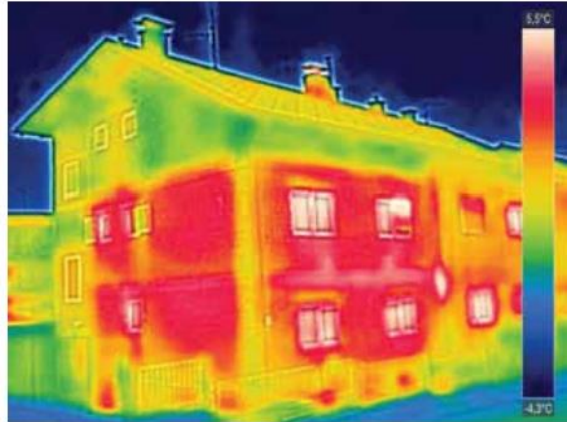
Figure 3.5. Thermal imaging of a home shows where heat is being lost. The red colour indicates a higher temperature which means those areas of the house are losing more heat to the outdoors. The yellow and green areas of the house are better insulated and lose less heat.
